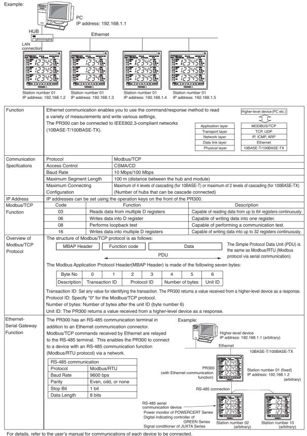
Note: If Ethernet communication is used, the RS-485 communication interface is used specifically for the Ethernet-serial gateway function. Therefore, it is not possible for a higher-level device such as a PC to access the PR300 via the RS-485 communication interface.
