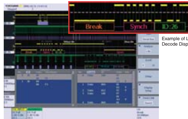
Example of simultaneous analysis and waveform (decode) display of CAN and LIN bus signals
