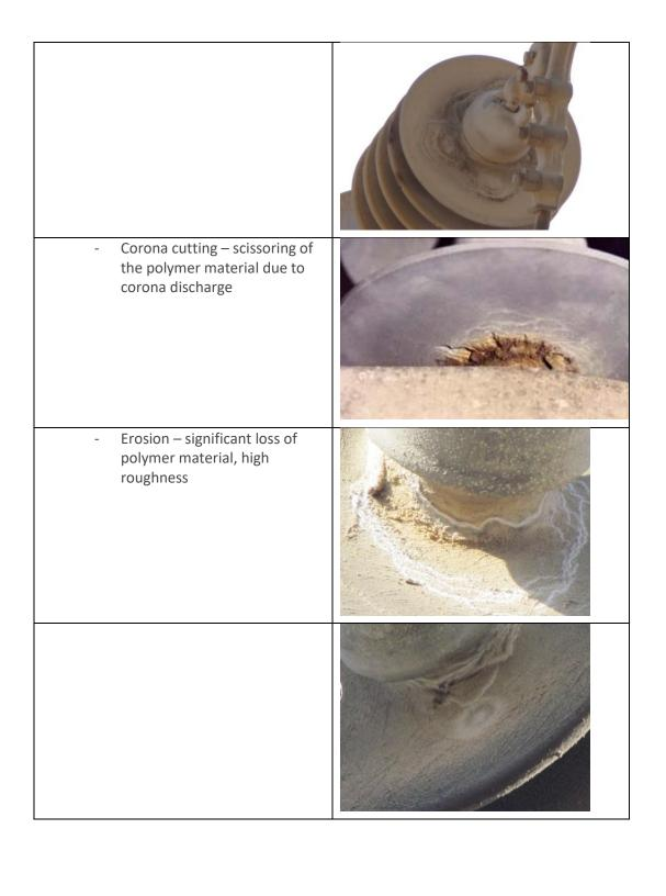
Rod exposure Power Arc damage – caused by high current or flashover Puncture - the polymer material is ruptured due to disruptive discharge occurring through the dielectric Cutting /splitting – tear, crack which reduces the creepage distance or the thickness of the sheath
