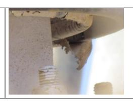
**Deteriorated insulators** - those with superficial ageing signs that will neither have a significant reduction in their performance nor represent any reliability risk. Although these conditions do not require replacement, utilities should monitor any deterioration.
