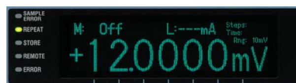
High resolution output with ±120,000 display counts and 100 nV steps minimum
