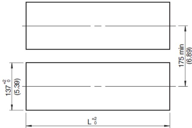
Side-by-side Mounting (vertically, max. 3 units)
