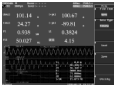
Example of inrush current measurement in an inverter-type cleaner
