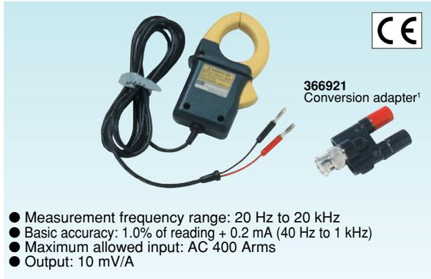
A separately sold adapter (366921) is required for connection to WT210/WT230. For detailed information, see Power Meter Accessory Catalog Bulletin 7515-52E. This model is treated as a special-order product.
