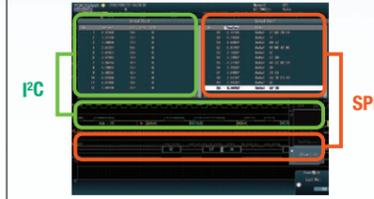
Many systems contain multiple serial buses. The DLM4000 analyzes two different serial-bus types simultaneously. A combination trigger of two different serial buses is also possible.
