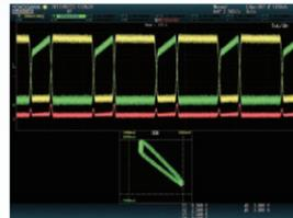
By dividing the long memory into segments, the SOA (safe operating area) can be analysed and, peak voltages between switching cycles can be compared by overlaying or one-by-one replay.
