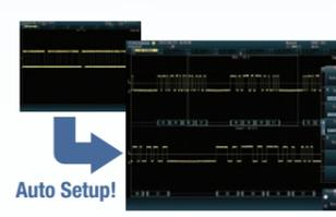
Intelligent serial-bus auto-setup feature enables quick and easy setup. The bit-rate and voltage thresholds are set automatically.
