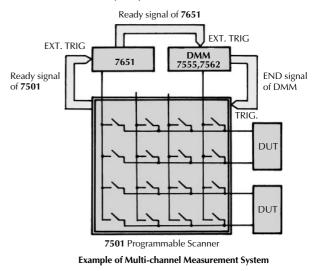
Evaluation test of amplifier DC characteristics can be made by supplying input signal to the amplifier from the 7651 and reading output of the amplifier by the DMM.
