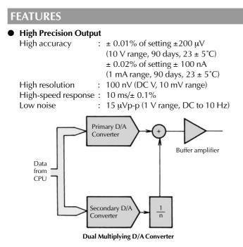
The 7651 uses multiplying D/A converter technology. Extremely high resolution is realized through the use of dual digital to analog converters. In addition, the linearity is further enhanced by software driven compensation technique.
