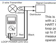
This is an example of a connection with a 2-wire transmitter. When the HART load resistance is ON with a loop power of 24 V, there is a load of up to 20 mA. Therefore, you can measure outputs of 4-20 mA while operating the 2-wire transmitter.
