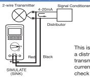
This is an example of a connection to a distributor used with a 2-wire transmitter. You can simulate (sink) current of an up to 48 V supply to check the loop circuit.
