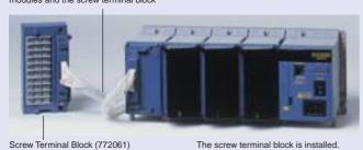
Detach the plate with clamp terminals from the MX110-UNV-M10 or MX115-D05-H10. Then, use the connection cable (772062) to connect the input module without the plate to the screw terminal block (772061).
