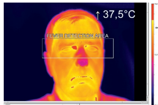
IR temperature measurement at the Medial Canthus for a close correlation to the core body temperature
