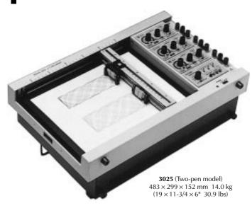
The 3025 is a fast, high-performance A4 X-Y recorder, available as a one- or two-pen model. Both models offer high slewing speed and high acceleration. The slewing speed and acceleration of the one-pen model in the Y axis is 2,200 mm/s 7.6 G, and 2,000 mm/s 5.1 G in the X axis.
