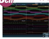
During the evaluation of a power supply design, it is necessary to measure noise, ripple, voltage margin and current, as well as timing margins and the jitter of the startup-shutdown sequences. As the number of waveforms in modern power supply designs is increasing, especially for intelligent digitally-controlled power supplies, battery management systems, and wireless power supply systems a four-channel oscilloscope is not enough.
