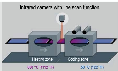
Construction of a glass tempering plant
