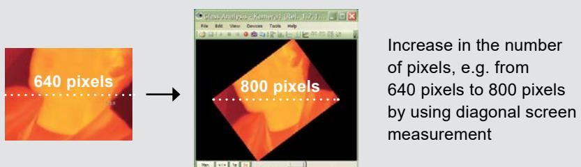
Increase in the number of pixels, e.g. from 640 pixels to 800 pixels by using diagonal screen measurement
