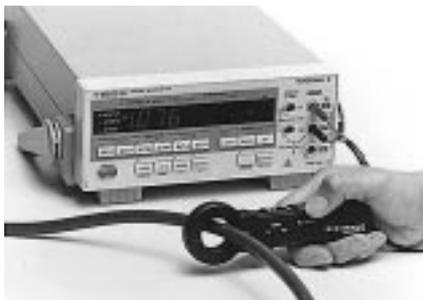
Current measurement using a current clamp (751106)
