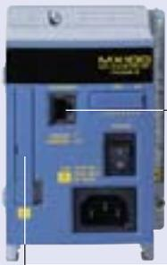
The main module is the engine that controls data acquisition. It is equipped with a power supply, an Ethernet port, and a CompactFlash card slot. **One main module can accommodate up to six input/output modules. The user can choose up to six modules of any type.**
