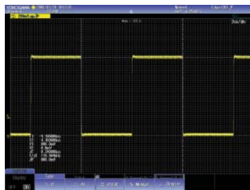
Simultaneous level and time difference measurement with the \Delta T \& \Delta V cursor
