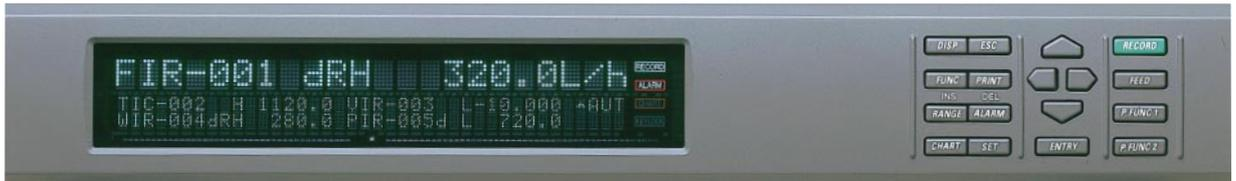
The large vacuum fluorescent display shows a total of 102 characters, one line of 22 large characters, and two lines of 44 smaller characters. It displays the measured results and alarm statuses in an eas-
