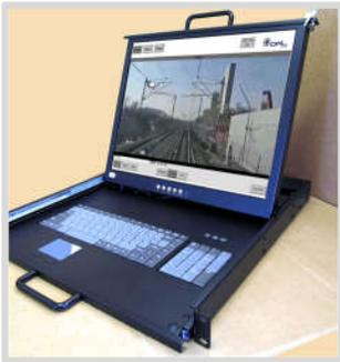
DayCor® Rail is a corona detection driven system dedicated to assist electrical railways management maintain ongoing safe operation of their mass transportation networks. **Rail combines monitoring, processing and reporting modules** that interact automatically to supply in real time information about the condition of overhead catenary systems.
