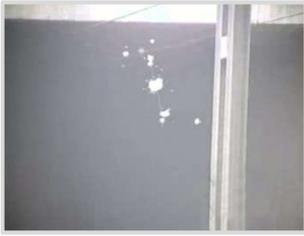
Broken strands, bird cages and any protruding elements on catenary OLE conductors have corona and are therefore captured and reported by DayCor® Rail. GPS data is stamped on the recorded images and enable finding on time the exact cases of fray conductors. To guarantee
