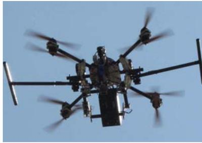
DayCor® Swift is a bi spectral UV-Visible block camera module with excellent scanning & corona detection capabilities, that fit monitoring of HV & MV electrical installations. Swift can be installed on a fixed mount or on a moving pan & tilt with 360° rotation or used on a UAS.
