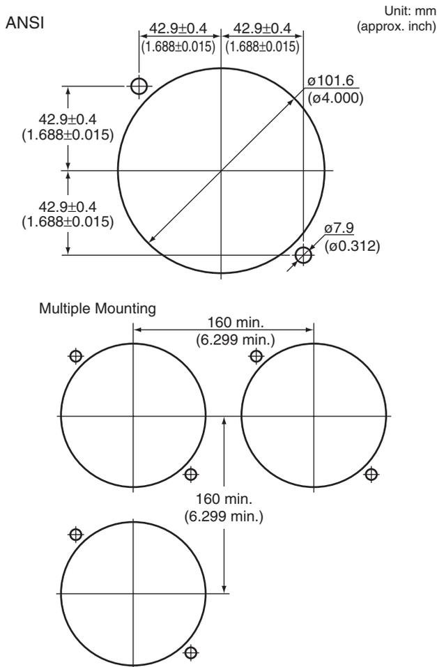
Normal Allowable Deviation= ±(Value of JIS B 0401-1999 tolerance grade IT18)/2
