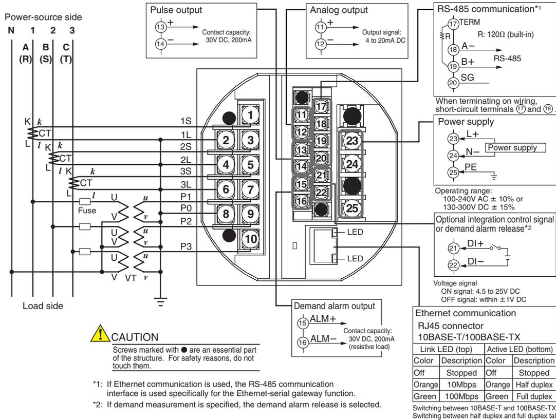
● Three-phase four-wire system (2.5 element)
