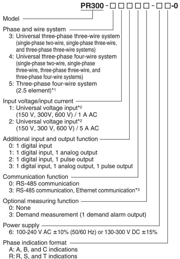
\*1 Can be used only when the voltage is in a state of equilibrium. The phase and wire system cannot be changed.
