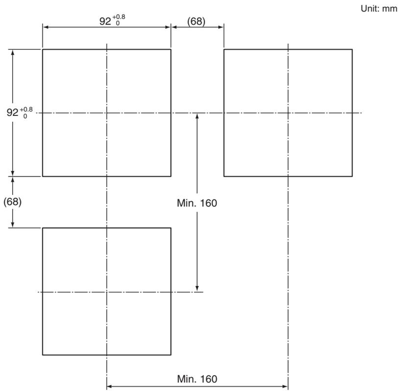
Normal Allowable Deviation=±(Value of JIS B 0401-1999 tolerance grade IT18)/2
